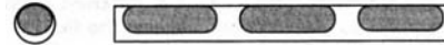
Fig. 2 Water-wedged rest configuration of oil slugs in water. This is promoted by small pipes, small density differences, large interfacial tension and hydrophilic walls (water-wet concrete walls, for example). Restart of this configuration is much easier than the restart of the completely stratified configuration shown in Fig. 1.
